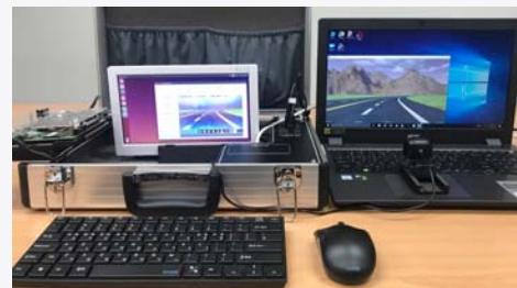
AD Emulation Platform (Hardware-In-the-Loop Platform)
